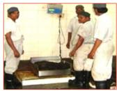
**Step 5: Weighing of Fleshed Hides:** Weighing of each hide to ensure right categorization of grades.
